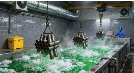
Pickling for rust removal
